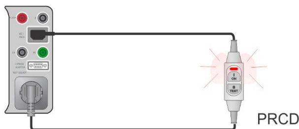
Figure 6.59: PE conductor (PRCD) test
