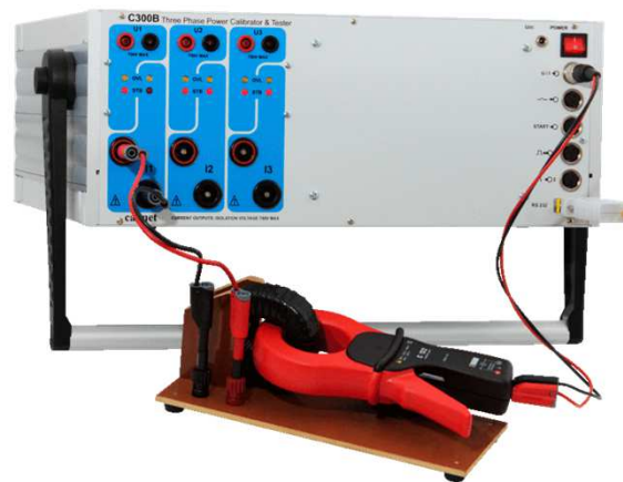
1000A clamp with 100 turns coil
