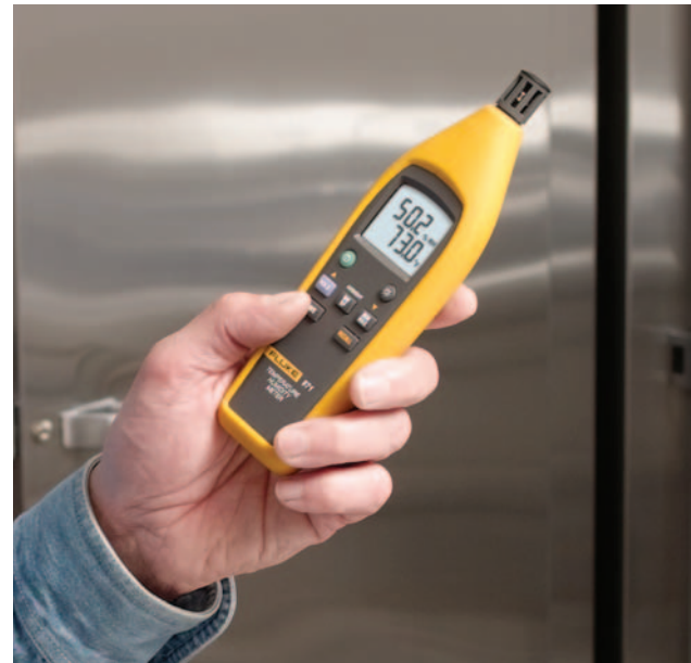
The Fluke 971 Temperature Humidity Meter measures temperature from -20 °C to 60 °C (-4 °F to 140 °F), dewpoint, wetbulb, and relative humidity from 5 % to 95 %.
