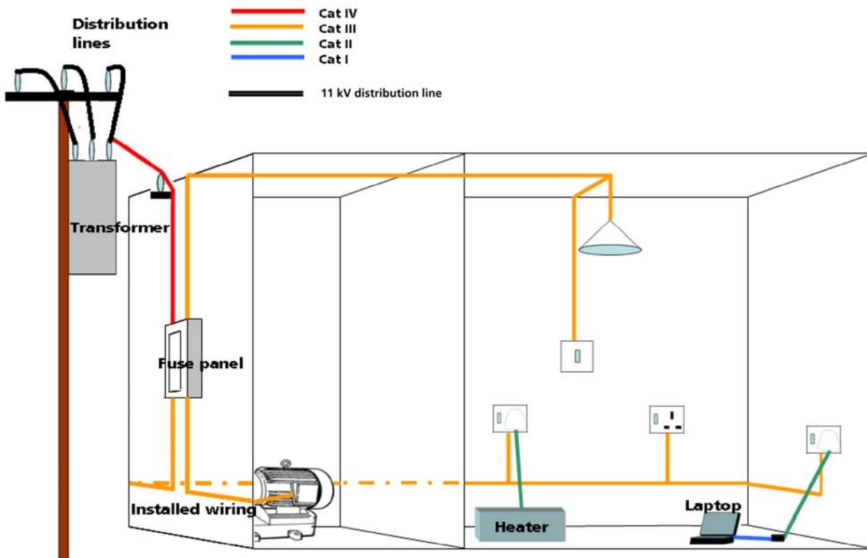
The picture shows the transmission lines (overhead or underground) as Category IV because the energy available from the supply and size of a transient is much higher near to the transformer. Test equipment suitable for use in this environment needs to be rated to CAT IV.
