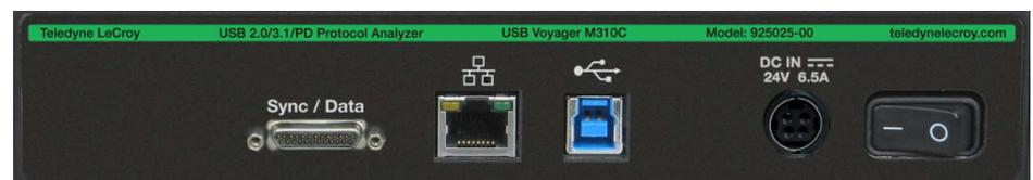
The Voyager M310C rear panel includes a Sync/Data port (used to cascade multiple systems, to CrossSync to other protocols and/or as an external signal input); 100BASE-T Ethernet and USB 3.0 ports (either of which can be used to connect to the host machine); a 24V DC input for power (from supplied adapter); and a power switch.
