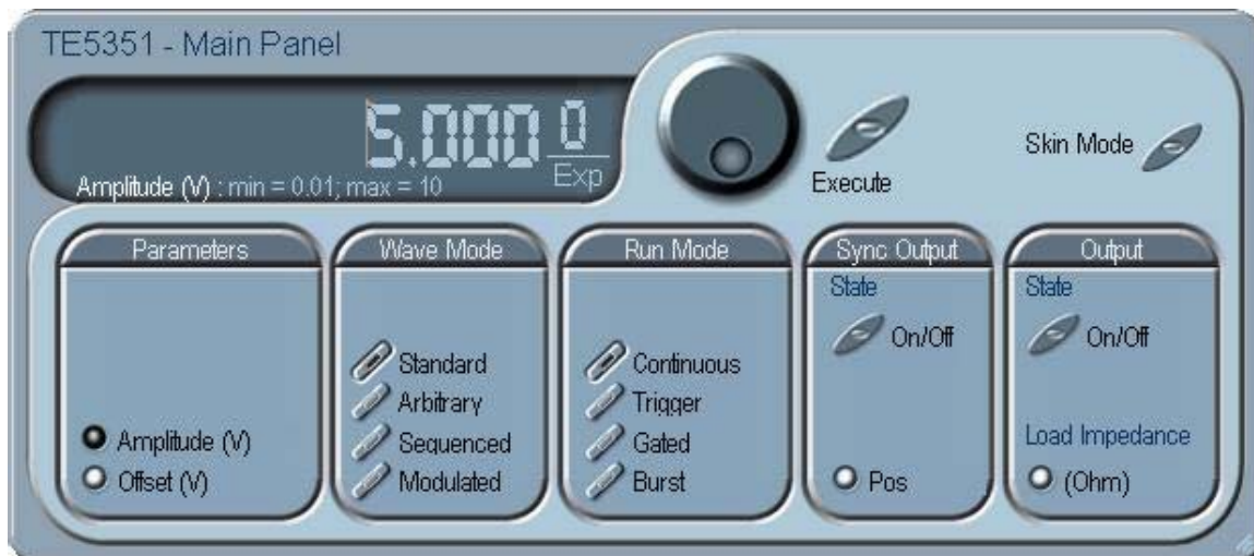
Figure 3-5, the Main Panel
