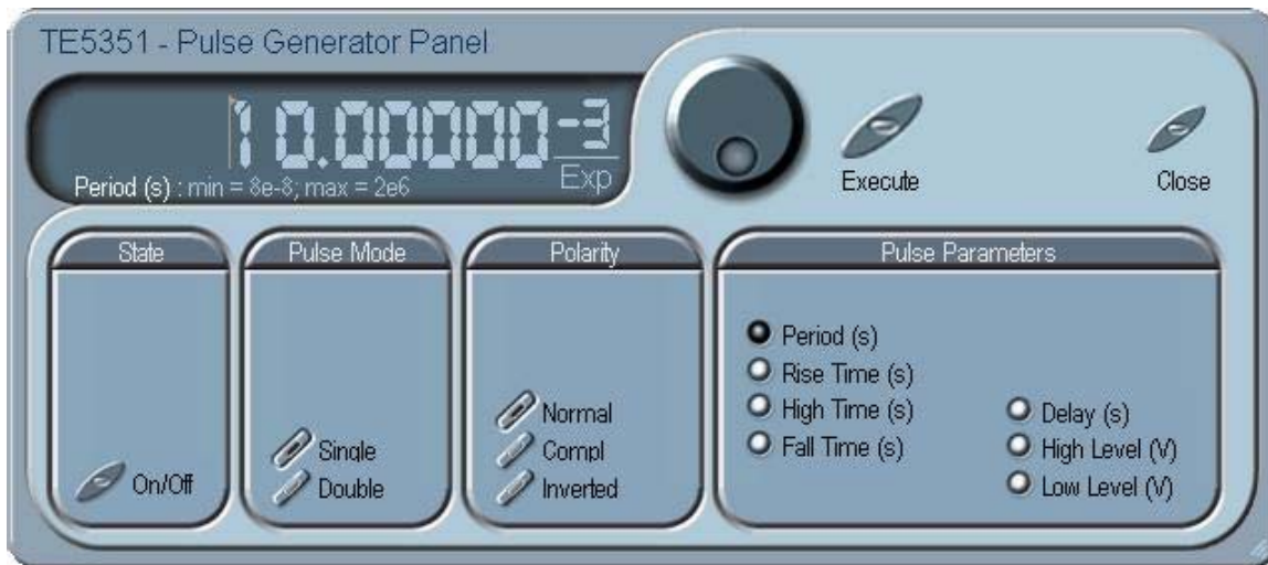
Figure 3-13, the Digital Pulse Generator Panel
