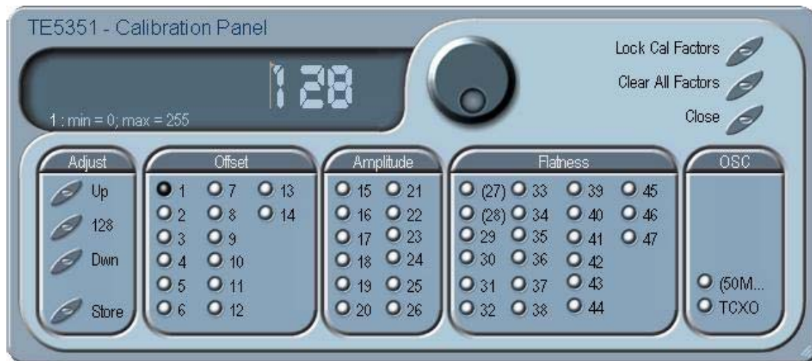
Figure 3-16, the Calibration Panel
