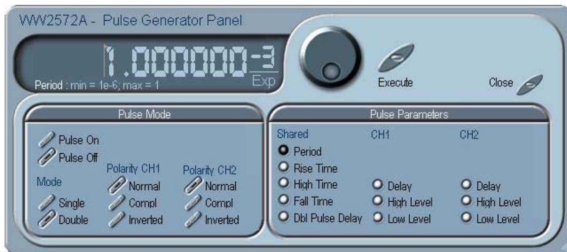
Figure 4-22, the Digital Pulse Generator Panel
