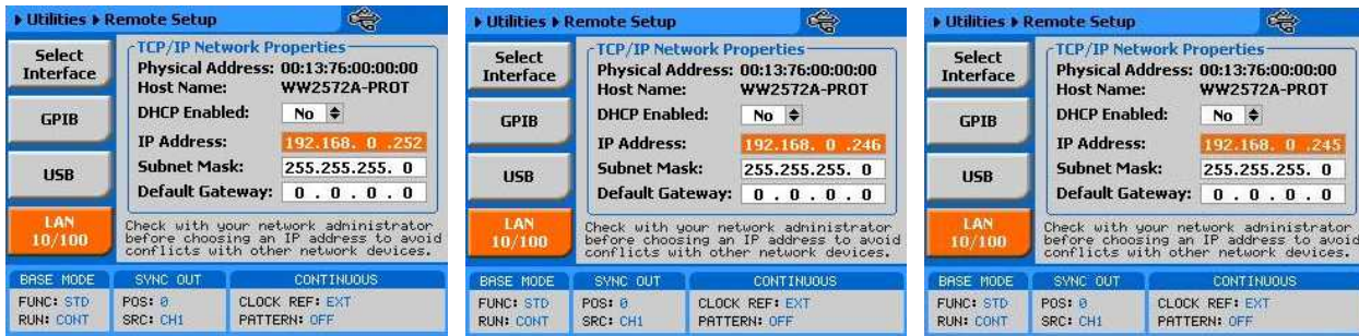
Figure 4-27, IP Address Setup Example (from left to right) Master and two Slaves
