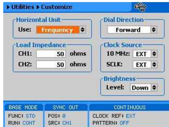
Figure 3-13, Modifying the SCLK and 10MHz Clock Source
