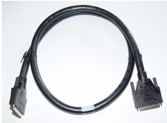
Figure 2-3, Digital POD Data Cable Example
