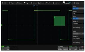
Isolate desired waveforms using up to two zone triggers. Touchscreen gestures allow users to generate zones by dragging a finger diagonally anywhere on the grid.
