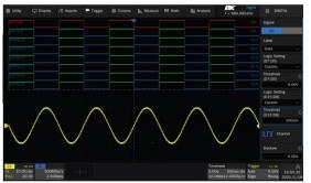
The MSO feature adds 16 digital channels allowing the acquisition and triggering of mixed signal waveforms.
