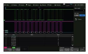
Serial bus decode supports I2C, SPI, UART, CAN, and LIN protocols. Information is displayed in tabular form.
