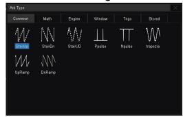
The built-in DDS waveform generator outputs waveforms with maximum frequencies of 50 MHz and ±3 V amplitude. Sine, square, ramp, pulse, noise, DC and arbitrary waveforms are available.
