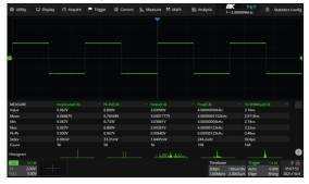
High speed waveform update rate displays infrequent glitches with excellent signal fidelity. Update rate can reach up to 500,000 wfms/s in sequence mode.
