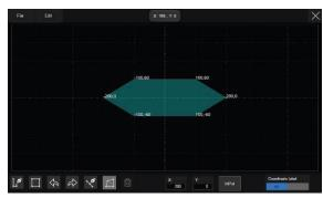
Use the built-in mask editor to create a mask and perform up to 80,000 pass / fail decisions per second. Failed frames can be stored as history frames for evaluation.
