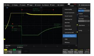
The power analysis tool can evaluate 11 different power supply or power device parameters such as power quality, inrush current and switching loss.
