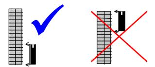
For 3 pin TO220 or TO92 packages, insert the IC in pins 6, 7 and 8 (lower left) of the socket with the metal tab or flat side facing to the right.
