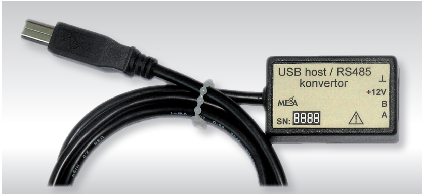
Fig. 1: USBhost/RS485 converter in version for MEg40*/supra and MEg202.2
