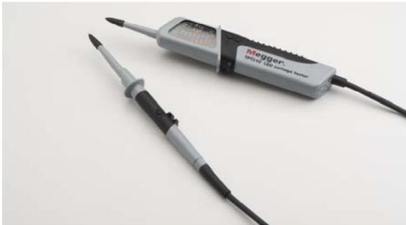
Electronic versions of the test lamp voltage tester are now very common and are generally divided into two variants. One has a LED ladder display that is divided into set voltages while the other has a LCD display that can display voltages in 1 volt increments. The ranges of these units are usually from 6 to 1000 V a.c. / d.c.
