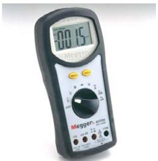
While most of these units are generally capable of indicating or even measuring voltages up to 1000 or 500 V a.c./d.c. they are not approved for confirming whether a circuit is live or dead because they do not have fixed test leads.
