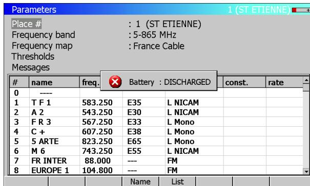
The battery is discharged; the appliance will automatically go off in a few minutes.
