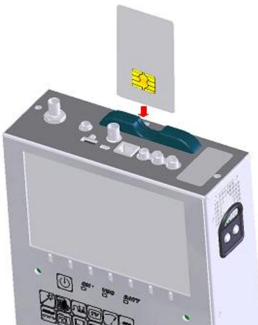
When displaying an encrypted channel, the processor checks if there is a user card and if the encryption mode is compatible.
