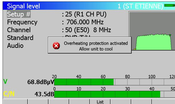
If the internal temperature in the appliance is over 60°C: change to protection mode.
