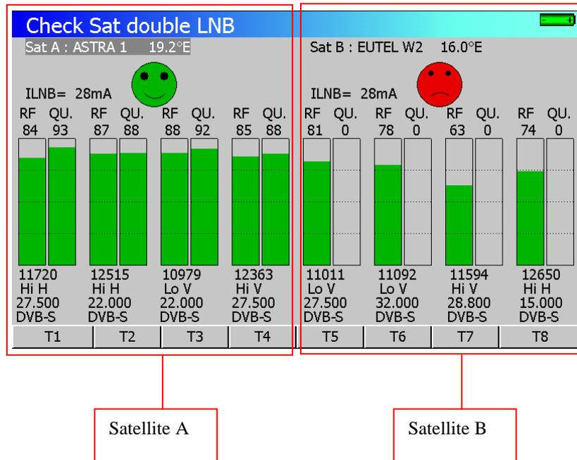
Satellite A is on the left side of the screen and Satellite B is on the right side.
