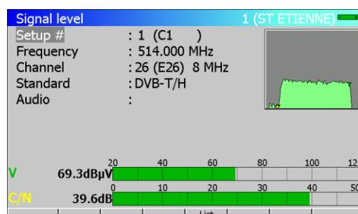
The level is indicated on a bargraph. A mini-spectrum is also displayed on this page.
