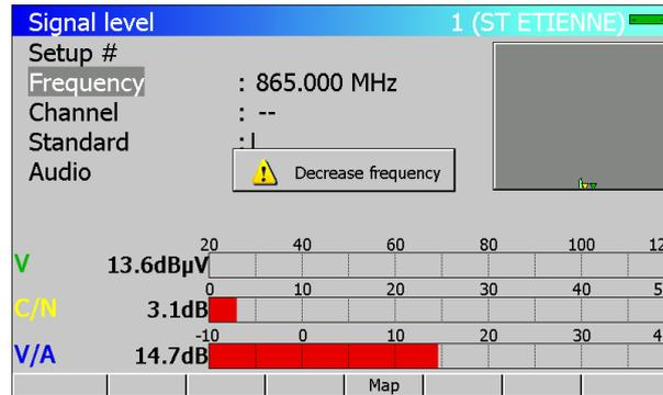
The appliance tries to perform a level measurement out of these possibilities (for example an Audio measurement with an 865 MHz video carrier).
