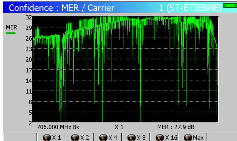
**Confidence** or MER/carrier represents the confidence rate for each carrier by the **DVB-T/H** DVB-T2 demodulator.
