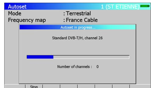
The appliance goes automatically to the **Measurement Map** mode when search is completed or when the user stops search.
