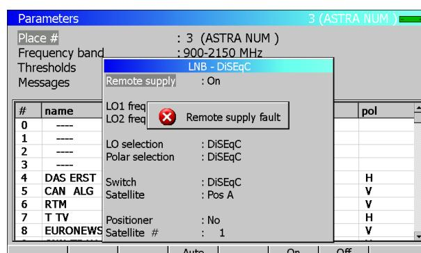
Remote supply fault: a voltage is already on the cable or current is already exceeding the maximum value.
