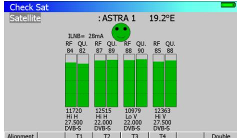
5/ select the satellite that you want to check (by using the sensitive rotary wheel).
