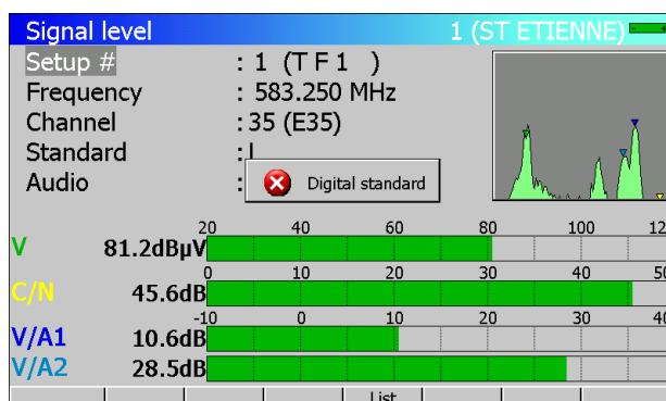
2<sup>nd</sup> press on the level key: The appliance tries to perform an error rate measurement with a **Standard** different **DVB-C, DVB-S, DVB-S2, DSS or DVB-T/H**.
