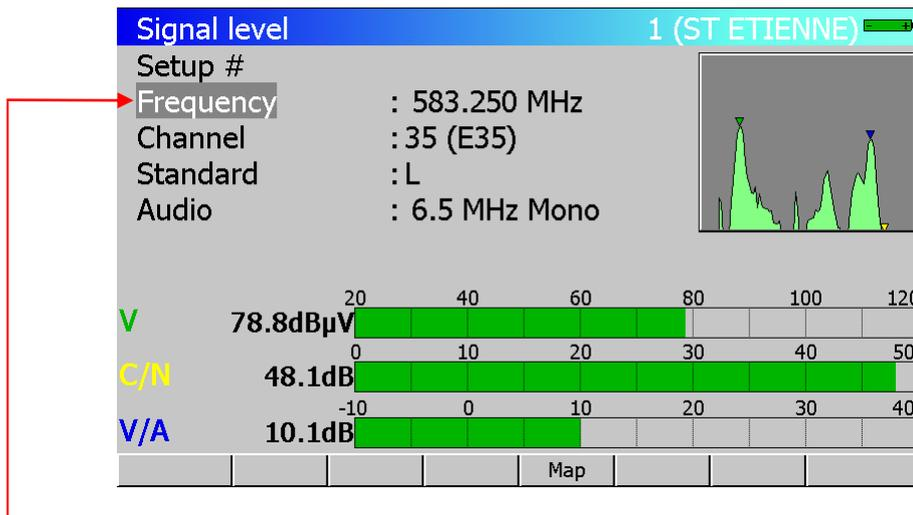
When a line is highlighted (reverse video) for a numerical parameter, use the sensitive wheel to modify the value.
