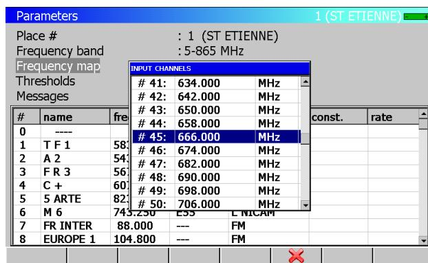
The **Frequency** of each **Channel** can be modified either by using the rotary wheel or by the keypad.
