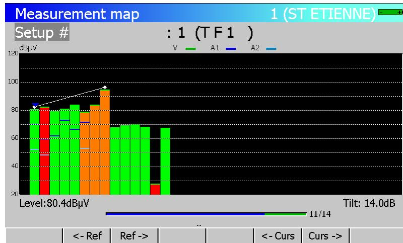
It is displayed in one screen; the histogram widths are automatically fitted according to the number of **Setups** included in the **Measurement map**.
