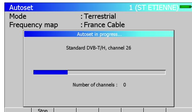
7/ once the search is completed, the appliance automatically goes to the Measurement Map mode. It displays different measurements (Level, MER...) for the found setups.
