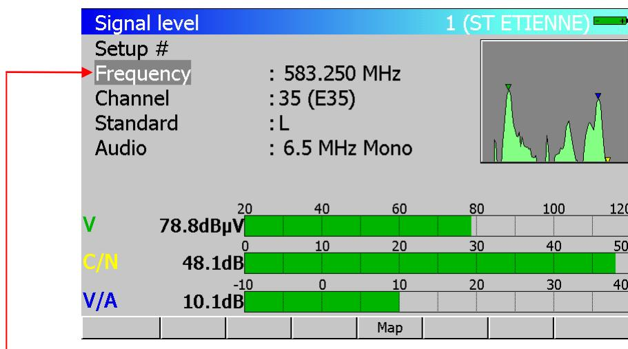
When a line is highlighted (reverse video) for a numerical parameter, use the sensitive wheel to modify the value.
