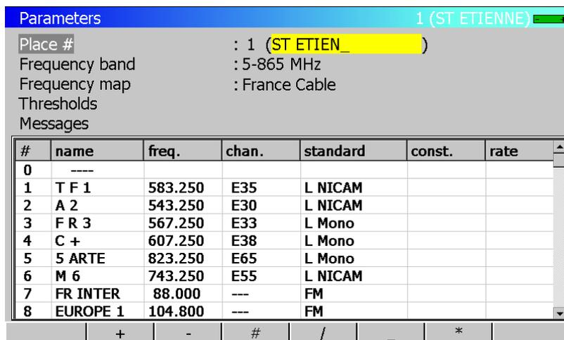
For some parameters you can enter alphanumerical data from the keyboard and the menu keys +, -, #, /, \_.
