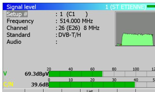
The level is indicated on a bargraphe. A mini-spectrum is also displayed on this page.
