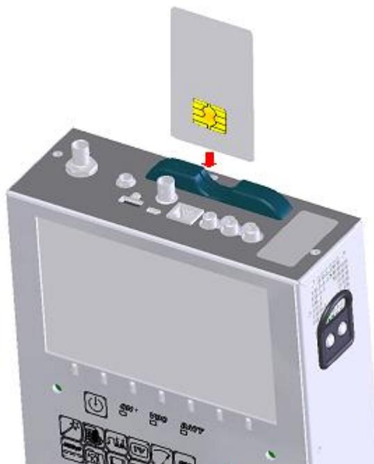
When displaying an encrypted channel, the processor checks if there is a user card and if the encryption mode is compatible.
