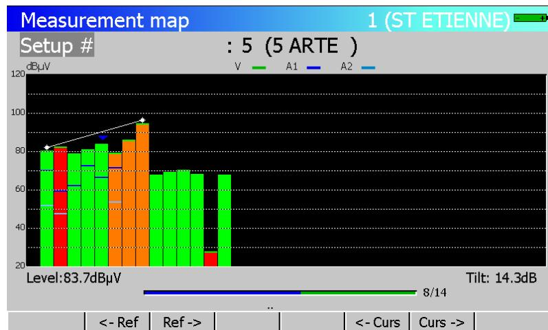
The **audio carriers**' levels are added on the associated video carrier histogram, according to the colours in the legend at the top and on the right of the page.
