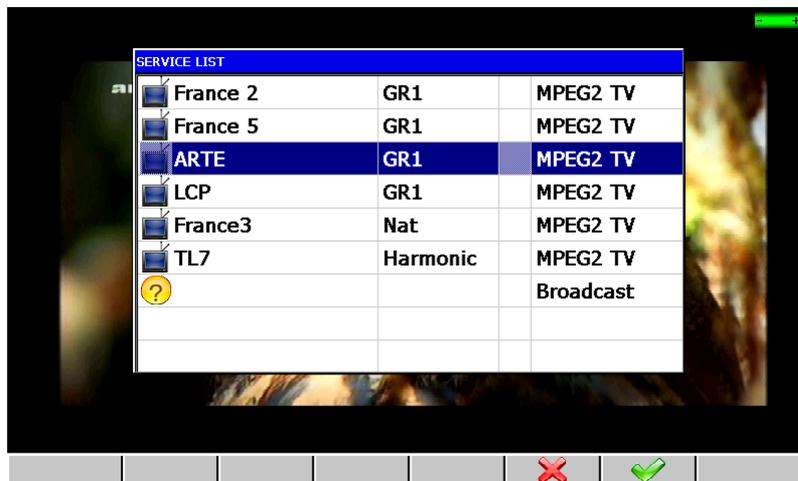
Choice of the service with the sensitive wheel or with the up/down direction keys.
