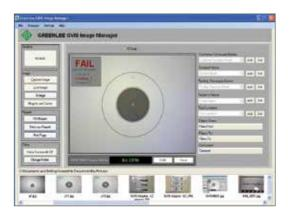
Figure 1 – Image showing automatic Pass/Fail analysis software
