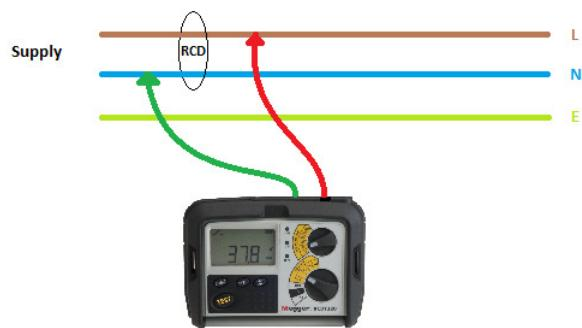
By connecting the RCD tester across the RCD on the phase and neutral conductors, the leakage current is then flowing through the test instrument so the RCD will still detect the imbalance of the current flowing. Although harder to make the connections, this is still a valid way of testing an RCD.
