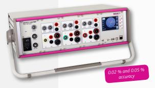
METES 340 REF provides high accuracy and a wide measuring range for precise measurements in single and three-phase applications.
