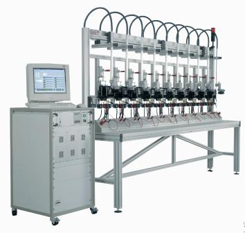
METES C meter test systems are fully automatic, multiple-meter test benches capable of testing and calibrating all types of electricity meters.
