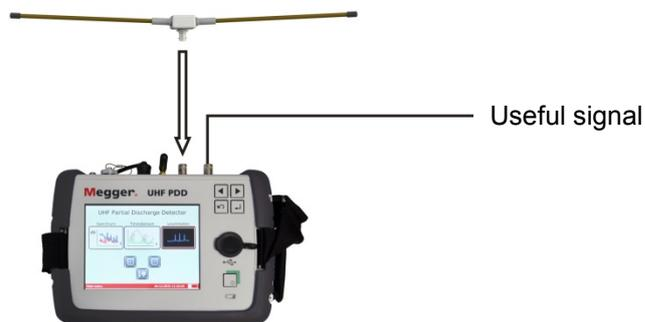
Instead of the reference antenna, a second sensor – as identical as possible in construction – can of course also be connected at the input **REF/RF/CAL 7** for comparison purposes:
