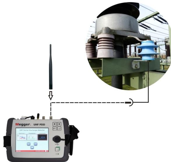
There is also the option of coupling the reference signal of a UHF reference antenna (e.g. of the supplied UHF dipole) at the input **REF/RF/CAL 7**.
