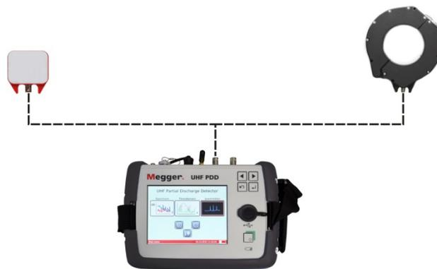
The connection of a comparison or reference sensor is not possible in RF mode.
