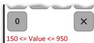
With **x**, the numeric keypad can be closed at any time, without adopting the entered value.
