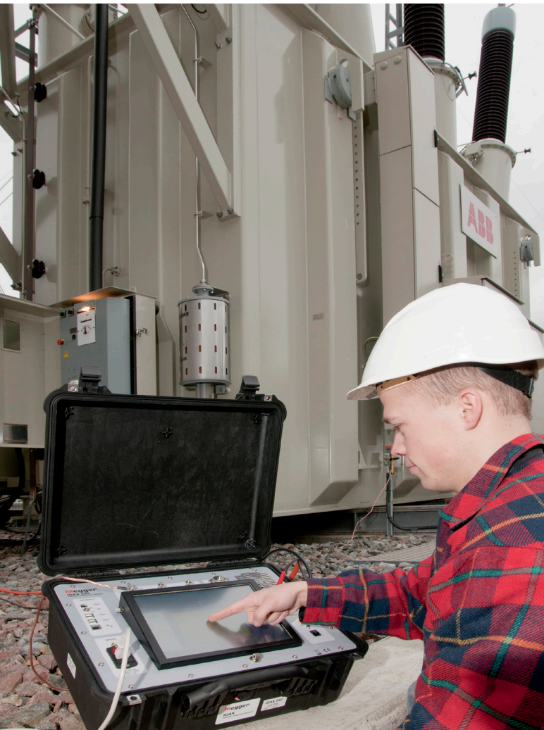
The IDAX 350 has a built-in computer but can also be used with an external PC.
