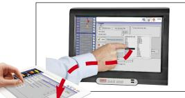
With Virtual Network Computing software, you remote control your DAS801 from a computer or a tablet.
