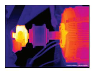
Identify a potential problem using a Fluke infrared camera.
