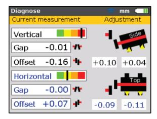
Corrective action using the Fluke 830 Laser Shaft Alignment tool.
