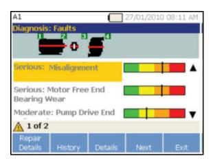
Diagnosis and repair recommendation using the Fluke vibration tool.
