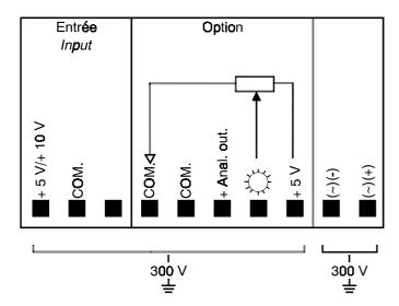
N.B.: For a negative scale range, reverse input polarity.
