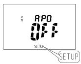
Setup the APO time from 1 to 60 minutes or OFF.
