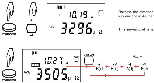
Reverse the direction of the current by pressing the ±I key and the instrument displays the average:  $\frac{R(+I) + R(-I)}{2}$
