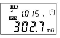
If the measurement is stopped by the disconnection of a clip, simply connecting it to another object starts another measurement, with no need to press the START/STOP key.
