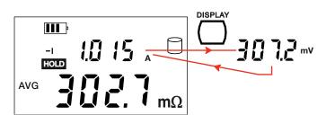
To display the voltage on the terminals of the resistance instead of the measurement current, press the DISPLAY key.
