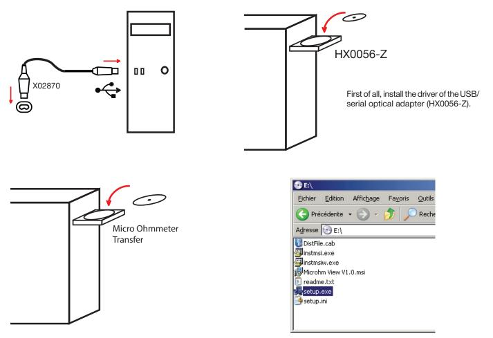
Then install the "Micro Ohmmeter Transfer" application software as explained in readme.txt.
