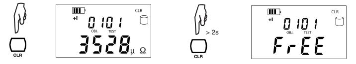
Use the arrows to select the test to be erased. The complete erasure of the memory is described in section 5.1.
