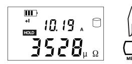
Once the measurement is over, it can be recorded. Press the MEM key.
