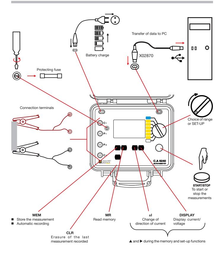
The C.A 6240 microhymmeter is a portable measuring instrument intended for the measurement of very low resistance values. It is enclosed in a site case and powered by a rechargeable battery with a built-in charger.
