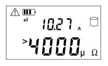
If the instrument indicates a range overshoot (> symbol), turn the switch to the next higher range and restart the measurement. Continue for as long as the range overshoot message is displayed.
