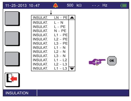
Using the ▲▼ arrows, select the type of insulation measurement you have just made and validate by pressing the OK key.
