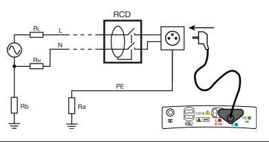
For a more accurate measurement of the fault voltage, plant the auxiliary rod at a distance of more than 25 metres from the earth electrode and connect it to the  $\mathbf{a}$  (R<sub>A</sub> S<sub>E</sub>) terminal of the device. The  $\mathbf{a}$  symbol is then displayed.
