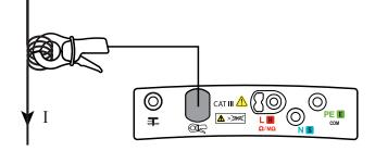
Here, the conductor passes through the clamp 4 times. You will have to divide the measured current by 4 to know the true value of I.
