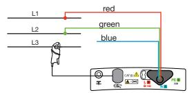
The power measurement can be made on different phases of an installation. This is why it has been made possible to index the recorded power value with one of the following values: 1, 2, or 3 (single-phase measurements on a three-phase network).
