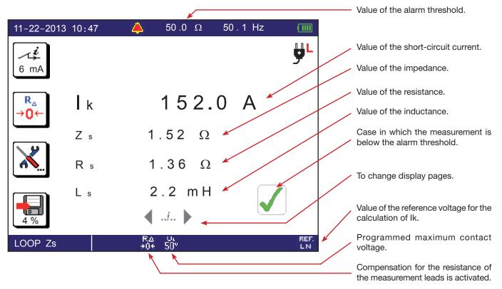
■ In the case of a measurement with tripping (TRIP) and without smoothing:
