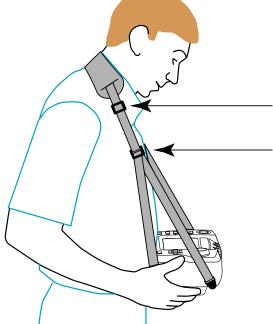
To withdraw the strap, slide a flat screwdriver under the tab of the fastener to lift it, then slide the fastener down.
