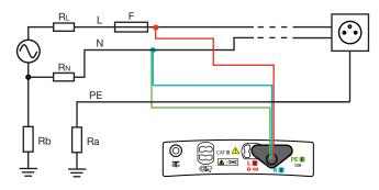
For the second measurement, connect the tripod cable to the instrument and to one of the outlets of the installation.
