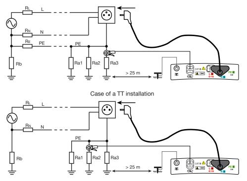
For a more accurate measurement, you can choose a high current (TRIP mode), but the RCD that protects the installation may trip.
