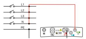
If the insulation is not sufficient, you must then make the measurement between each of the pairs to locate the fault. It is for this reason possible to index the recorded value with one of the following values:
