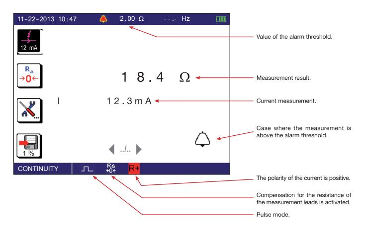
In the case of a resistance measurement  $(k\Omega)$ , there is no current reversal and no compensation for the measurement leads.
