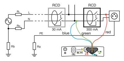
If it is active, the alarm on the tripping time informs the user by an audible signal, that the measurement is outside the range limits, so there is no need to look at the display unit.
