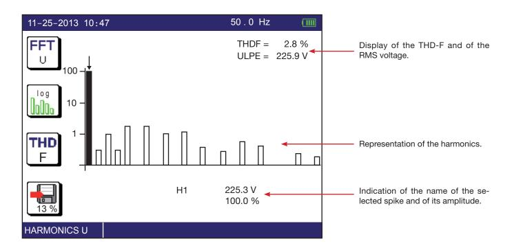
The frequency and amplitude of the selected harmonic (in black) are indicated at the bottom of the graph. To select another harmonic, use the  $\blacktriangleleft \triangleright$  keys. The device then shifts from the fundamental (H1) to harmonic H2, then to harmonics (H3, H4, ..., H25). And on the next page it sweeps the harmonics from H26 to H50.
