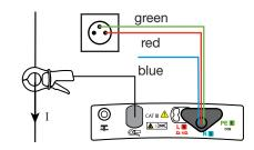
The current measured by the clamp is too high. Use a clamp having a higher ratio.
