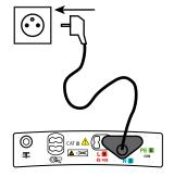
In the Zs ( $R_A/S_{EL.}$ ) and RCD, settings, the device also indicates the position of the phase on the display unit using the  $rac{P}{P}$  symbol. The mains socket outlet of the measuring cable is marked with a white reference spot.
