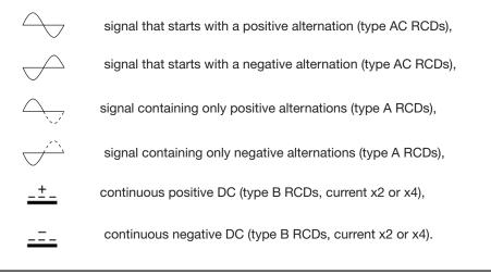
Depending on the type of fuse and the form of the test signal, only some values of the pulse current are possible.
