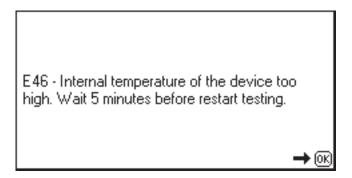
The internal temperature of the device is too high. Wait for the device to cool off before making another measurement. This case concerns essentially the test of residual current devices.
