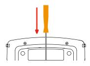
2. Turn the device over and insert a screwdriver into the hole in the battery pack.
