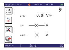
If  $U_{_{\text{N-PE}}}$  does not display – x --, the protection in the N terminal has been activated.
