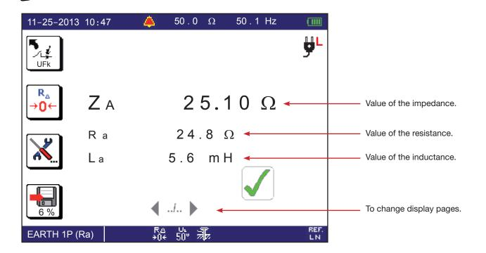
The third page displays the values of  $Z_s$ ,  $R_s$ ,  $L_s$ . The fourth page displays the voltages  $U_{LN}$ ,  $U_{LPE}$ ,  $U_{NPE}$  and on the rod ( $F_{LN}$ ) before the measurement.
