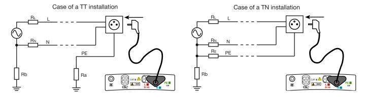
For a more accurate measurement, you can choose a high current (TRIP mode), but the RCD that protects the installation may trip.
