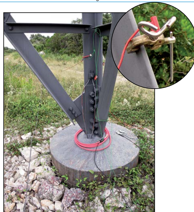
By using AmpFLEX™ sensors, you can measure on any pylon configuration.
