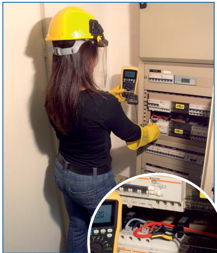
The sensors' flexibility is an advantage on industrial and domestic switchboards.
