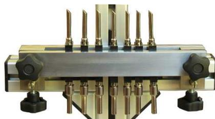
Spring contact pins of the EH20 are used to make connection to the meter and may be easily moved sideways and fixed in any desired position with distance between two adjacent contact pins from 14mm. It is also easy to remove and switch the pin positions for preparing the contact pin configuration to many different meter connection schemes, including single and three phase meters.
