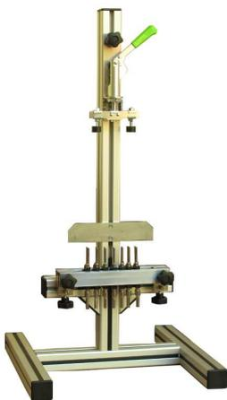
**Meter Suspension Rack with Quick Connection Device** – it enables electricity meters to be mounted and connected rapidly for the purpose of their adjustment, test and verification. Thanks to the smart design of the EH20 quick connection device, it may be used for the connection of practically all types of electricity meters with currents up to 100A. The quick connection device is fixed to the suspension rack by using of two knobs.
