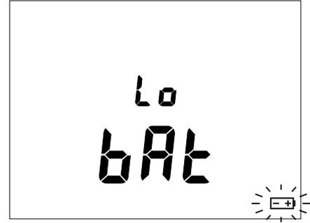
The batteries must then be replaced (see § 4.2)), since the battery life indication is no longer reliable.
