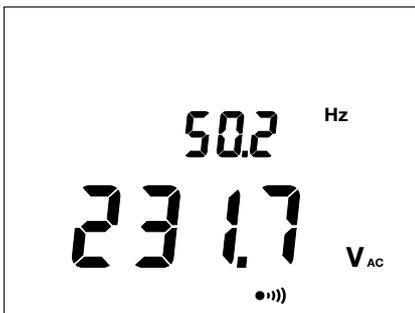
In the **MΩ** settings, the
