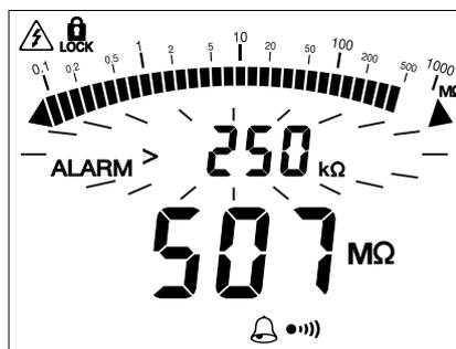
In the example above, the user can thus check that their continuity measurement is indeed less than 2 Ω, just by listening, without looking at the display unit. They can check insulation quality in the same way.
