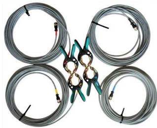
X winding test cable set
