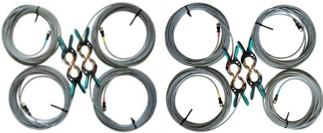
H winding test cable set
