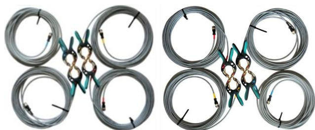
H winding test cable set
