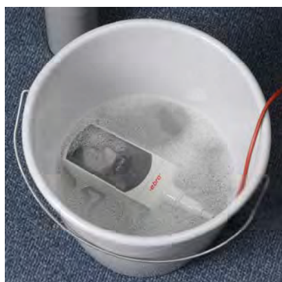
TF 410 - still working, thanks to IP 67
