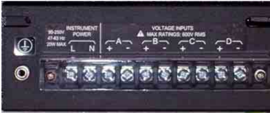
Figure 10 Terminal strip housed inside the terminal block assembly
