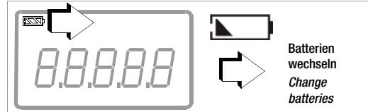
**Batterietausch – Battery Replacement**
