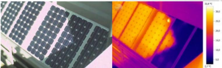
*Shaded Cells or Cells Concealed by Contamination*
