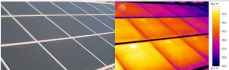
*Not Every Hot Spot is a Defect – Thermograph of the Junction Boxes*
