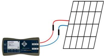
Connect the PROFITEST PVsun test instrument to the module with the help of suitable solar plugs.
