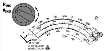
Read the measured value from the lower voltage scale 2.
