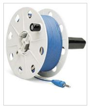
50m measurement cable coilded around a plastic drum. Connection to one end of the cable is accomplished with a jack which is integrated into the drum. The other end is equipped with a banana plug. The drum axle with handle can be removed for space saving storage.
