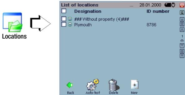
Individual locations included in this catalog can be supplemented or deleted. The hierarchy levels can be opened up by pressing the “+” symbol.
