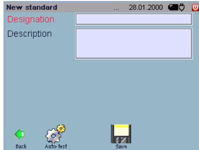
You can create a standard, i.e. its designation, upon which your tests are based. The designations included in this catalog can be used when a test sequence in accordance with a given standard is created.
