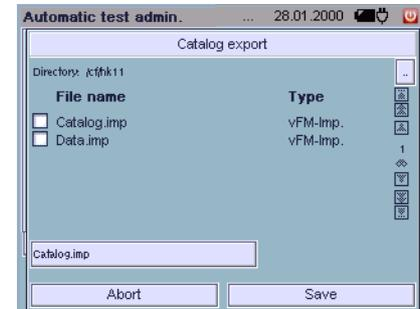
Data records are selected here for export to vFM / PS3 at the PC. Select the file in L&H Format function to this end. The respective file name ends with the .imp extension.
