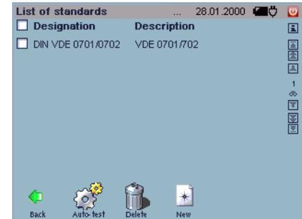
The designations for standards included in this catalog can be used when test sequences are created.
