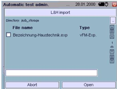
Lists or catalogs (e.g. designations) from various PC applications can be made available to the **test system** for test sequences using the import function.
