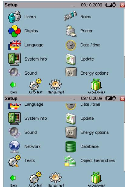
All of the settings which are required for operation and of the **test system** and the user interface can be entered in the setup menu.
