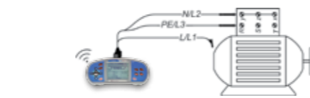
Test circuit for continuous resistance measurement
