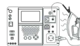
Touch leakage current test for Class II device
