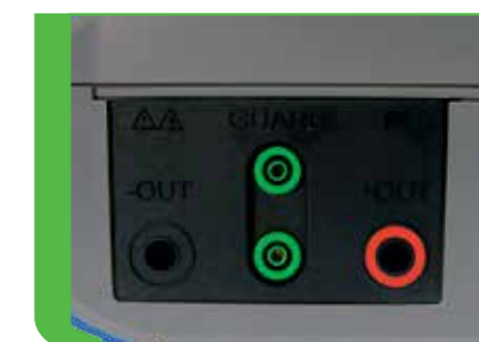
Guard terminal for connecting shielded test leads
