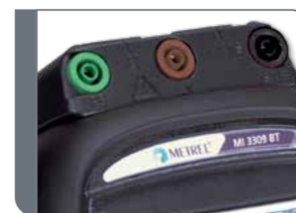
Inputs for testing fixed appliances.
