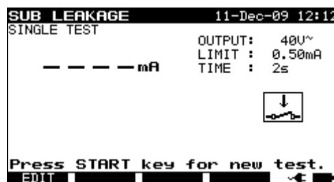
Sub leakage menu
