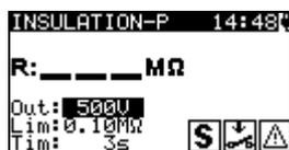
Figure 5.10: Insulation resistance - P menu
