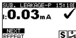
Figure 6.28: Substitute leakage - P result screen
