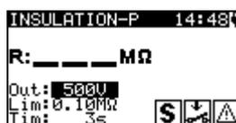
Figure 6.25: Insulation resistance - P starting screen
