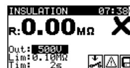
Figure 5.9: Examples of Insulation resistance measurement results
