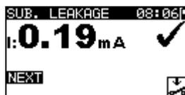
Figure 6.24: Substitute leakage result screen
