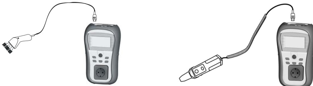
Figure 6.16: Connection of the barcode reader and RFID reader/writer
