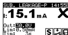
Figure 5.18: Example of substitute leakage - P current measurement results
