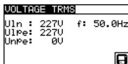
Figure 5.24: Voltage TRMS test result
