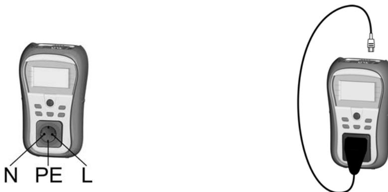
Figure 5.20: Polarity test of IEC cord
