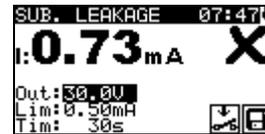
Figure 5.15: Example of substitute leakage current measurement results
