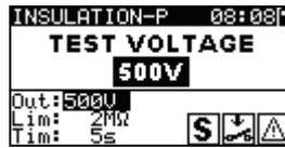
Figure 6.9: VDE Organizer autotest – Insulation resistance - P starting screen
