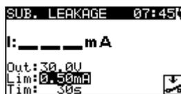
Figure 6.23: Substitute leakage starting screen
