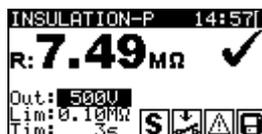
Figure 6.26: Insulation resistance - P result screen
