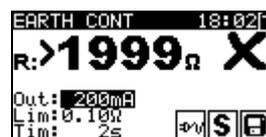
Figure 5.6: Examples of Earth continuity resistance measurement results
