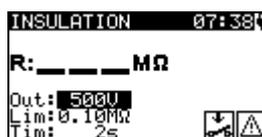
Figure 6.21: Insulation resistance starting screen
