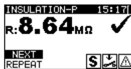
Figure 6.10: VDE Organizer – Insulation resistance - P result screen
