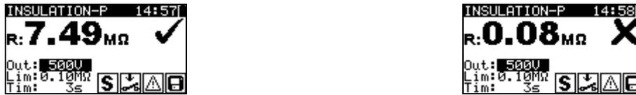
Figure 5.12: Example of insulation resistance - P measurement results
