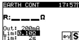
Figure 5.2: Example of single test measuring menu
