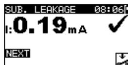
Figure 6.8: VDE Organizer – Substitute leakage result screen
