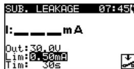
Figure 5.13: Substitute leakage menu
