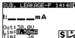
Figure 6.11: VDE Organizer – Substitute leakage - P starting screen
