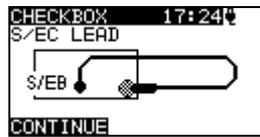
Figure 4.16: S/EB test lead check starting screen
