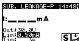
Figure 6.27: Substitute leakage - P starting screen
