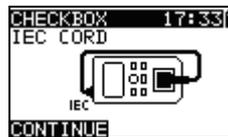
Figure 4.17: IEC test cord check starting screen
