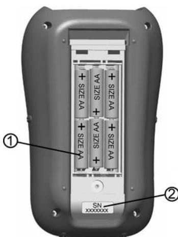
Figure 2.4: Battery compartment
