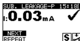
Figure 6.12: VDE Organizer – Substitute leakage - P result screen
