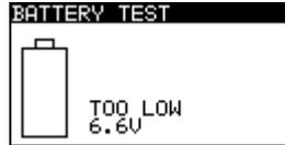
Figure 1.1: Discharged battery indication
