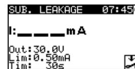
Figure 6.7: VDE Organizer – Substitute leakage starting screens
