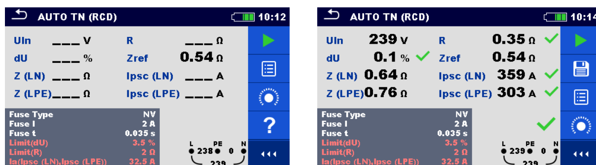
Figure 8.8: Examples of AUTO TN (RCD) measurement results
