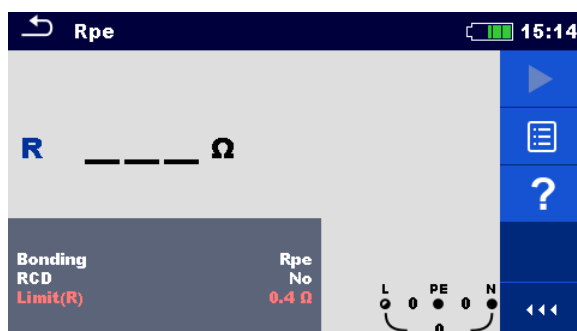
Figure 7.74: PE conductor resistance measurement menu
