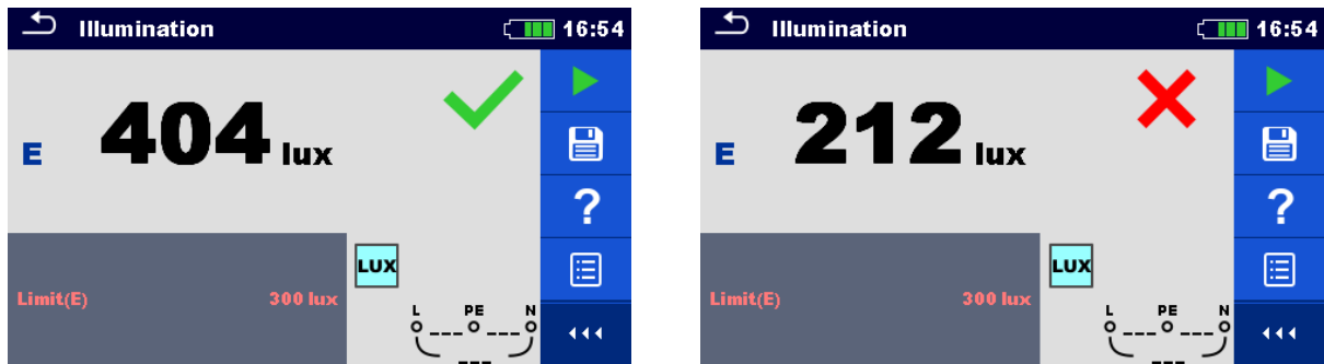
Figure 7.79: Examples of Illumination measurement result
