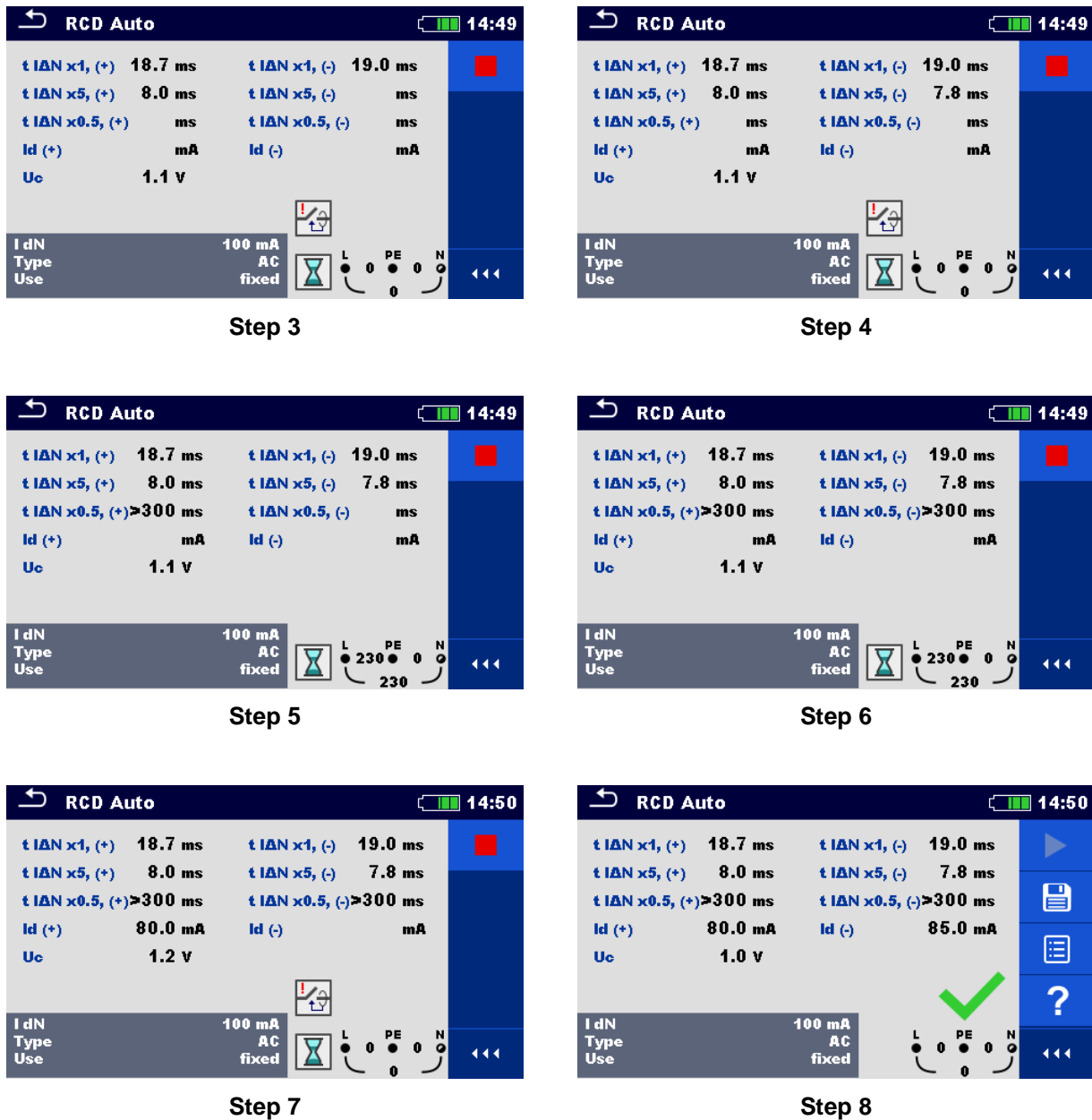
Figure 7.27: Individual steps in RCD Auto test
