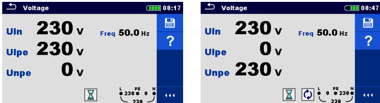
Figure 7.4: Examples of Voltage measurement in single-phase system
