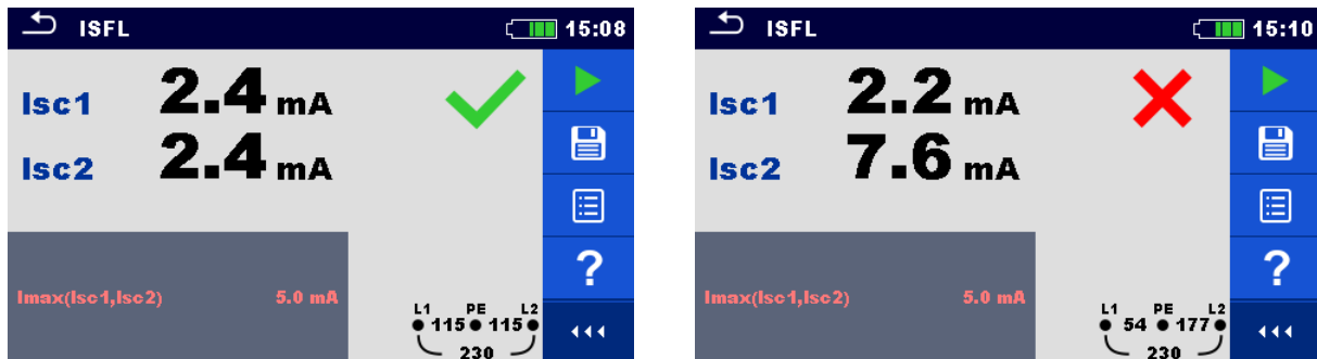
Figure 7.70: Examples of First fault leakage current measurement result
