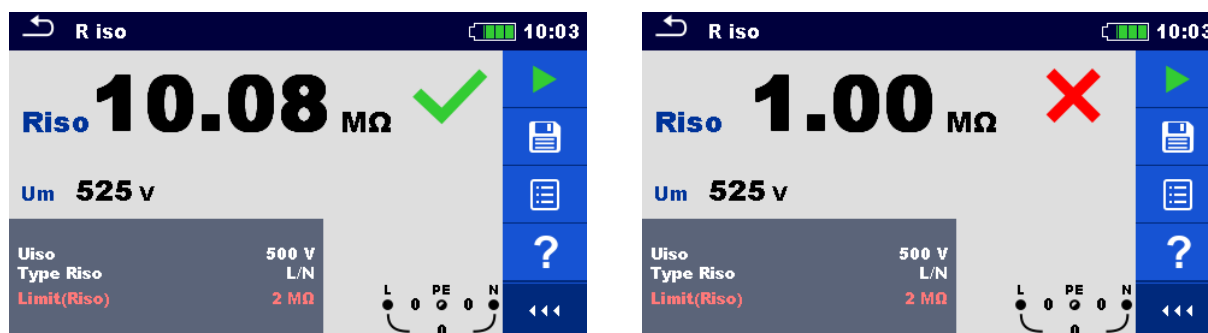
Figure 7.9: Examples of Insulation resistance measurement result
