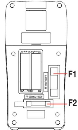
For safety reasons this fuse must always be replaced by an identical model:
