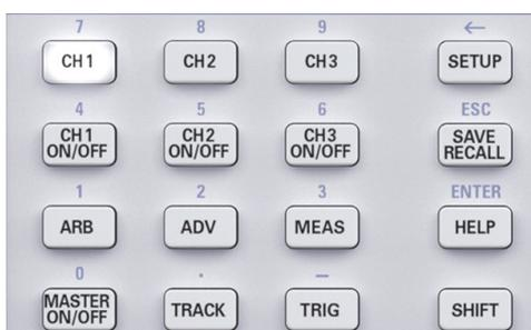
Fig. 4.2: Numeric keypad with function keys
