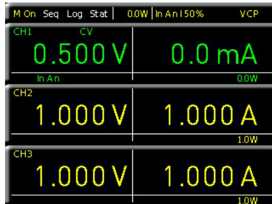
Fig. 6.4: Analog In example
