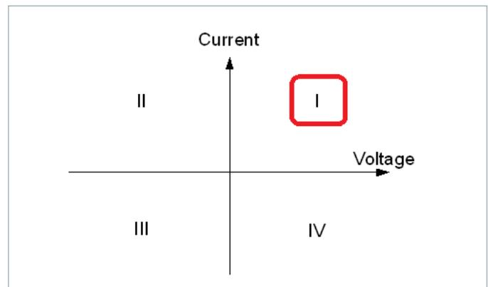
Fig. 6.10: Power supply quadrants diagram
