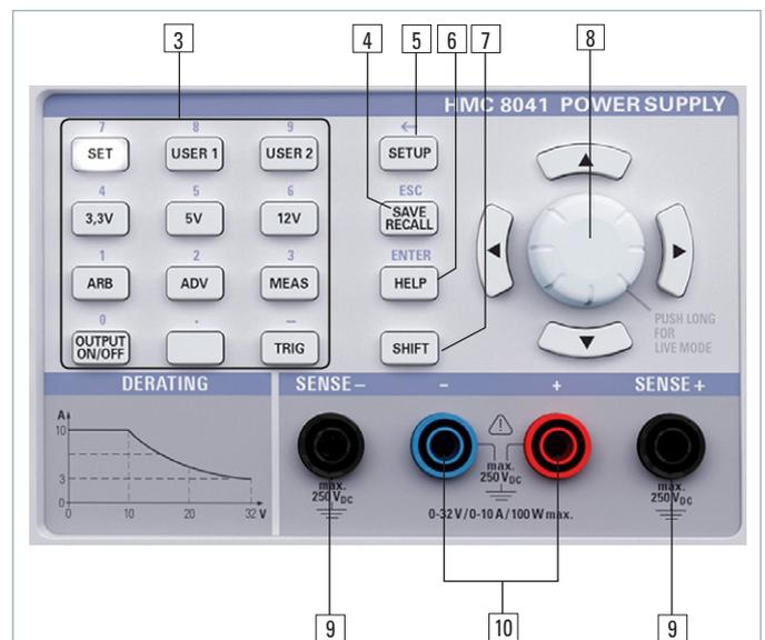
Fig. 2.4: User panel R&S®HMC8041 (1 channel instrument)
