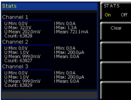
Fig. 6.12: Statistic example R&S®HMC8043
