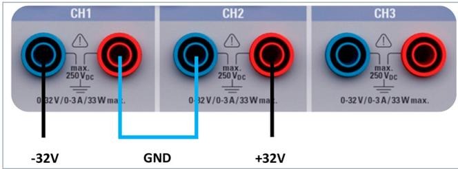
Fig. 6.11: R&S®HMC8043 connection
