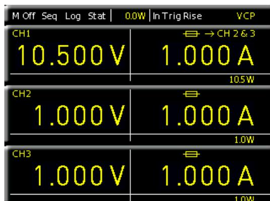
Fig. 5.4: Fuse Linking example
