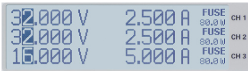
Fig. 5.1: 1-V position for all three channels (R&S®HMP2030)
