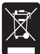
Fig. 1.4: Product labeling in accordance with EN 50419
