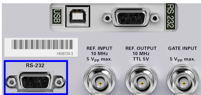
Fig. 2.2: Instrument back panel HM8134-3
