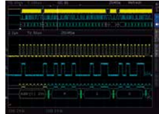
SPI bus signal, MISO / MOSI decoded
