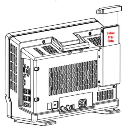
4. Replace the cover, then push in the knob and turn it clockwise to tighten it.
