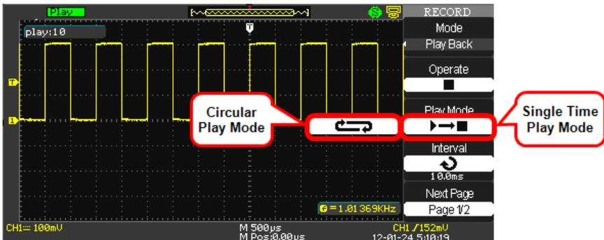
3. Press the **Interval** option button and use the **Adjust** front panel knob to dial in the desired interval between record frames for the playback of your recorded waveforms.
