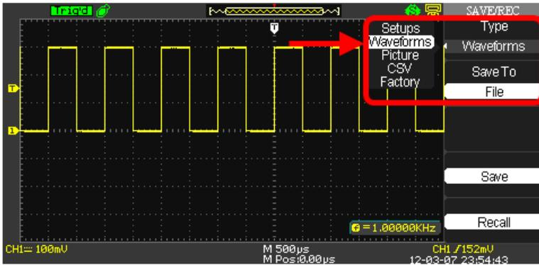
2. Press the **Type** option button and select **Waveforms**.
