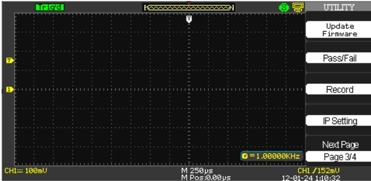
1. Press the **Update Firmware** option button to update the oscilloscope using the USB memory device. For more information, see the **Updating the System Software** (on page 82) section.
