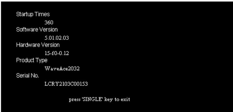
**NOTE:** As indicated, press the **SINGLE Front Panel** (on page 7) button to exit the System Status screen.
