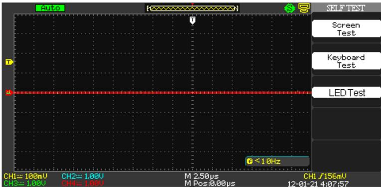
2. Choose from Screen, Keyboard, or LED tests by pressing the respective option button.
