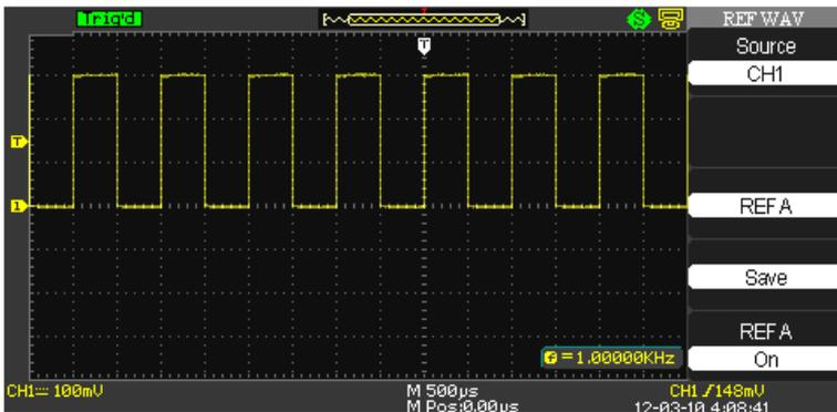
2. Press the **Source** option button to select the input signal channel.
