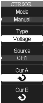
2. Cursors are placed according to the cursor measurement Mode - **Manual**, **Track**, or **Auto** – chosen in one of the following manners:
