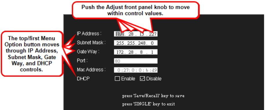
Use the top/first Menu Option button to move through **IP Address**, **Subnet Mask**, **Gate Way**, and **DHCP** controls. Push the **Adjust Front Panel** (on page 7) knob to move within a control and turn the knob to change values.
