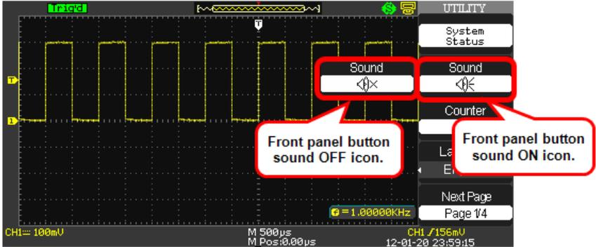
3. Turning the Frequency Counter On/Off shows or hides it from the grid display.
