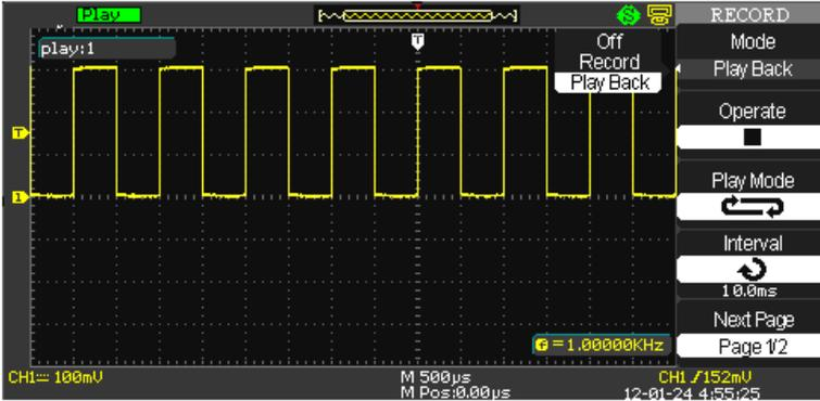
1. Press the Operate option button to **Start/Stop** playback.
