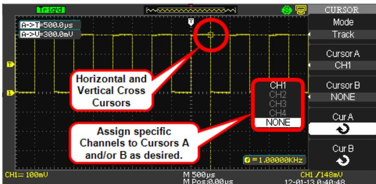
Adjust the cursor position on the waveform by turning the **Adjust** front panel knob. Measurements are shown in the upper-left of the grid.
