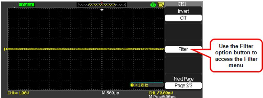
4. Press the **Filter** option button and select **On**.
