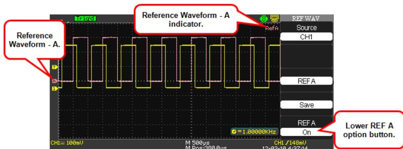
This also shows or hides the reference waveform from the grid display area. Now, you can make adjustments to your waveform leaving the REF A trace intact for comparison. There's also a reference waveform indicator shown on the upper-right of the grid display.
