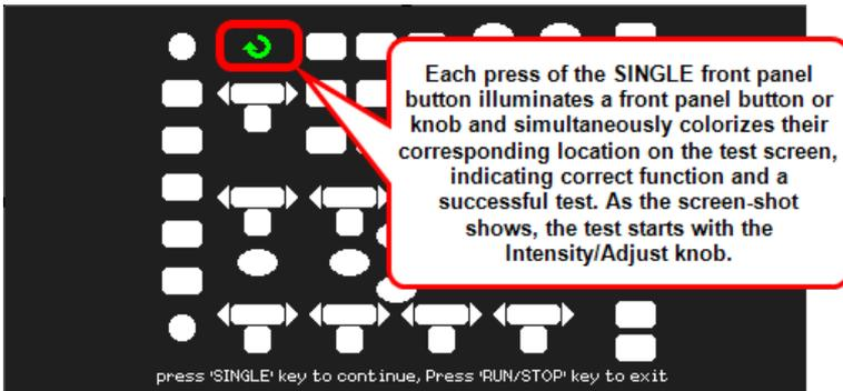
*LED Test - Each press of the SINGLE front panel button illuminates a front panel button or knob and simultaneously colorizes their corresponding location on the test screen, indicating correct function and a successful test. As the screen-shot shows, the test starts with the Intensity/Adjust knob. Test as many LEDs as desired. As the screen indicates, press the RUN/STOP front panel button to exit.*
