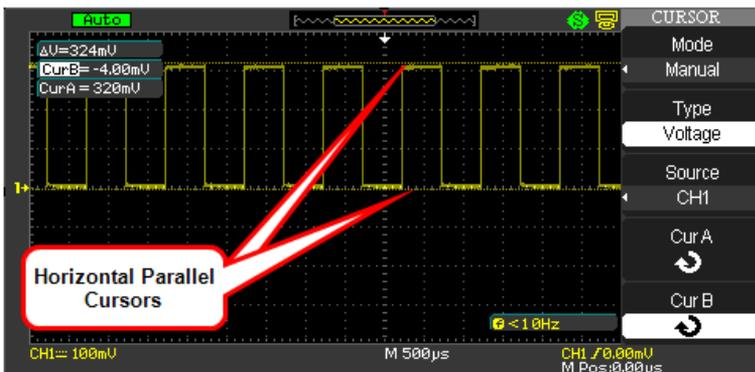
Voltage cursors appear as horizontal lines on the display and measure the vertical parameters. Time cursors appear as vertical lines on the display and measure the horizontal parameters.
