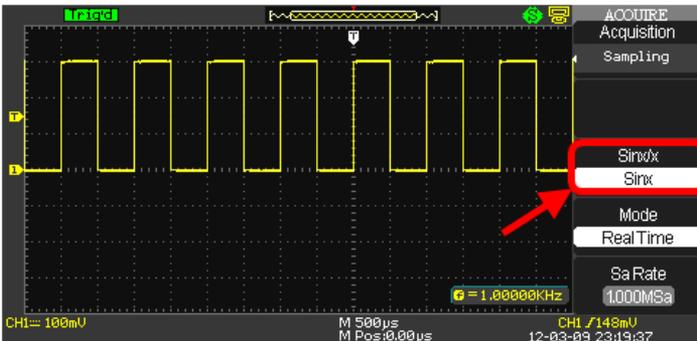
Sinx/x interpolation is suitable for reconstructing curved or irregular wave shapes, especially when the sample rate is 3 to 5 times the system bandwidth.
