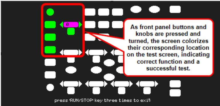
*Keyboard Test - As front panel buttons and knobs are pressed and turned, the screen colorizes their corresponding location on the test screen, indicating correct function and a successful test. Test all of the instruments buttons and knobs as desired. As the screen indicates, pressing the RUN/STOP front panel button three times exits the keyboard test.*
