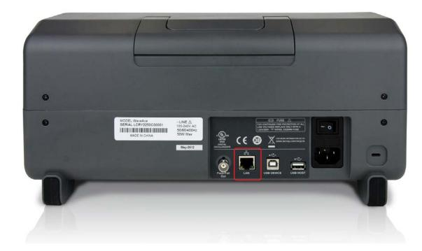
1. Attach an Ethernet cable from the LAN port on the rear of the scope to an Ethernet port on the controller machine or a connection device on the same network as the controller.
