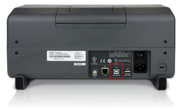
2. Install NI-VISA on the controller machine. NI-VISA contains the USB drivers needed to form the interface between the oscilloscope and the controller. NI-VISA can be downloaded free from <u>www.ni.com/visa</u>. You may use either the NI-VISA run-time or the full download. The run-time download is significantly smaller.
